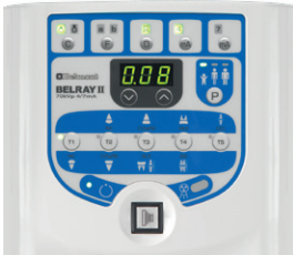
Keypad control panel with single-piece membrane
