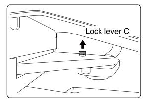
① Pull the lock lever C on the swing arm bracket, then swing the light pole slightly to chair legrest side.
