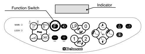
• The contents of display on the indicator on the doctor membrane switch panel change sequentially each time when the function switch is pressed to select a desired setup. Contents and sequence of function switch setup are described below.
