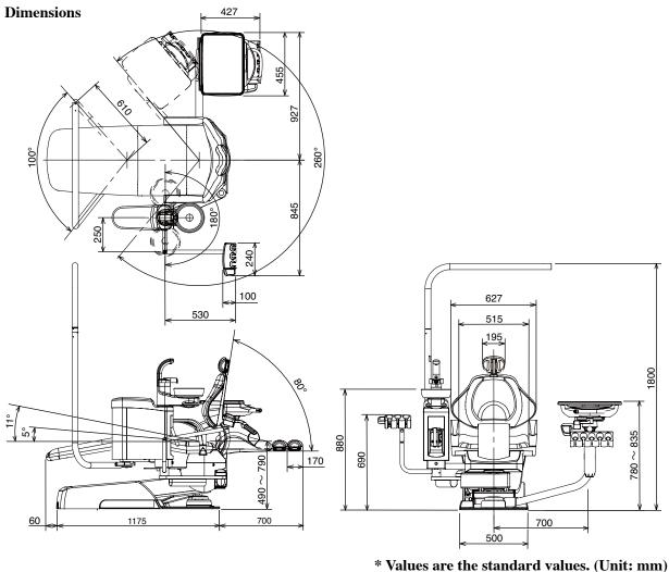
Values are the standard values. (Unit: mm) Dimensional tolerance:  $\pm 10\%$
