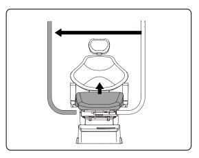
(2) Lift the toe board of seat cushion and swing the light pole to other side as shown on the left figure.
