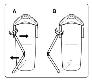
(3) After moved the light pole, the balance arm position become A position as shown on the left figure. Adjust the position of the balance arm to position B as shown on the left figure.
