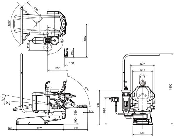
\* Values are the standard values. (Unit: mm) Dimensional tolerance: ±10%
