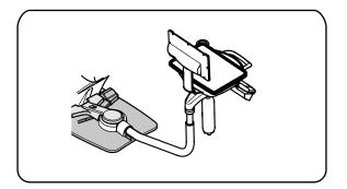
When the doctor table is turned to the back side of the backrest and chair auto motion of the chair is locked
