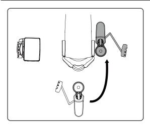
(8) Swing the cuspidor unit and the assistant holder as shown on the left figure. When the cuspidor unit moved to correct position as shown on the left figure, the lock lever A on the swing bracket can be locked automatically.
