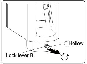
(9) Turn the lock lever B to change the position of hollow to down side. Move the cuspidor unit in left or right lightly until make sure the lock lever B is return to lock position.
