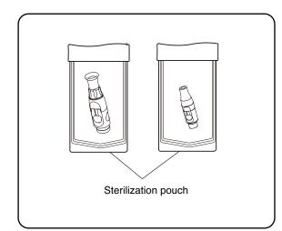
■ Sterilization of vacuum / saliva ejector handpiece
