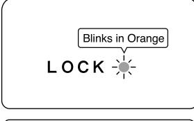
The safety mechanism that inhibits chair motion works while of the following actions is taken. The "LOCK" LED indicator lamp is lit in orange in this state.
