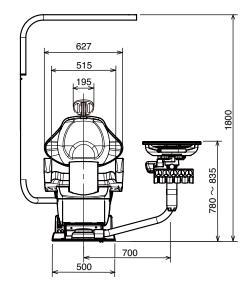
\* Values are the standard values. (Unit: mm) Dimensional tolerance: ±10%
