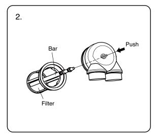
2. The filter can be removed from solid collector by pushing the bar from front side of the solid collector and clean with running water.
