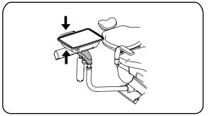
If excess pressure (upward or downward) is applied to the doctor table by the movement of chair, safety device stops the chair movement to protect the table from being damaged.
